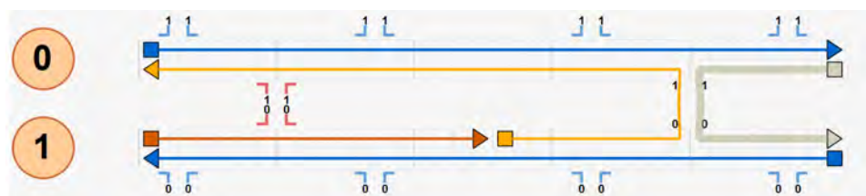
Figure 12: A close-up of the path panel with the example two helix structure, showing staple crossover locations (RED) and scaffold crossover locations (BLUE).
